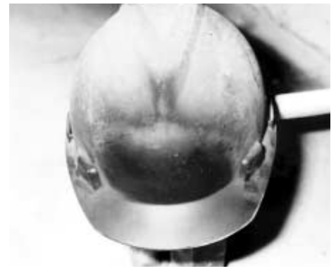
The hardhat that saved a worker's eyesight.
