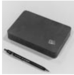
Bricks of magnetized strontium ferrite, stacked inside permanent magnets in the 8-GeV Line and Recycler, create the magnetic field.
