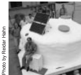
A prototype surface detector developed at Fermilab.
