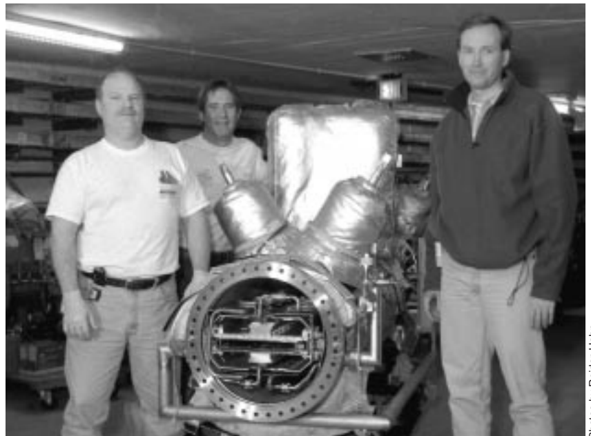
Dan Poll, Jim Budlong and Paul Derwent with the Accumulator stacktail upgrade stochastic cooling pickup tank.
