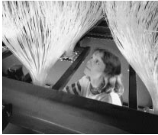
The HyperCP experiment used optical fibers in their 64-layer sampling calorimeter. 256 fibers guide light from the calorimeter to one cell containing a photomultiplier. Casey Durand, now assistant professor at the Maricopa County College District in Phoenix, Arizona worked on the installation of the fibers in 1996.
