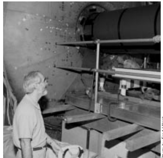
A crane maneuvered the tracker into position with the detector (left). Task manager Del Miller lined it up with the DZero solenoid (center). Gaston Gutierrez watched as the tracker slid slowly into place at the heart of the DZero detector (right).
