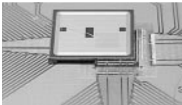
This sensor, about 9 millimeters long, contains 18 columns of 160 silicon pixels each. Using bump-bonding, a prototype of the first-generation pixel read-out chip developed at Fermilab is attached from below.
