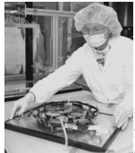
The F-disk is a high-precision detector used inside the DZero detector to identify particle tracks. Lead technician Sharon Austin has been responsible for mounting the wedge-shaped silicon components.
