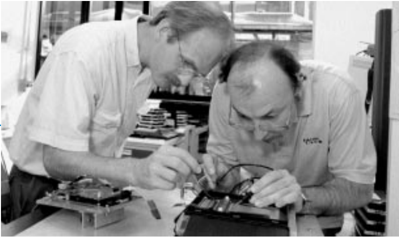
Fermilab's Marcel Demarteau (left) and Mikhail Merkin, Moscow State University, test the electronics of a wedge-shaped microstrip sensor, a critical component of the DZero silicon detector.
