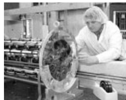
Jim Fast prepares the central silicon for transport. The detector wraps around the DZero beam pipe, with a clearance of about 1.8 mm.
