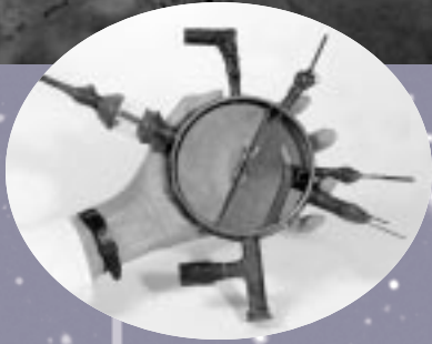
This cyclotron (above), built in 1930, accelerated protons in a spiral motion to 80,000 electron volts. Fermilab's Tevatron (top), 4 miles in circumference, accelerates protons to more than 12 million times that energy.
