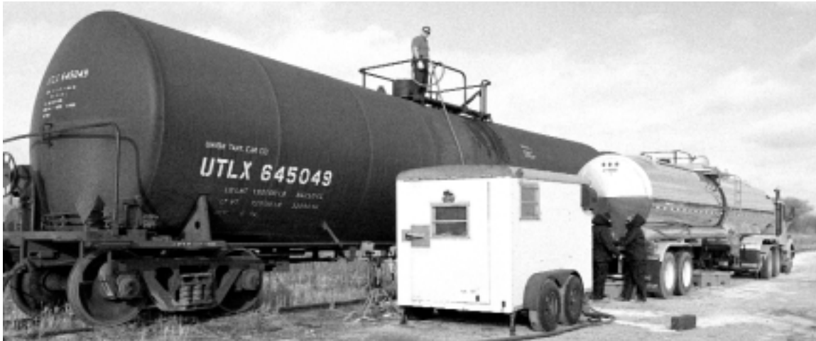
Oil for the MiniBooNE detector arrives at Fermilab by railcars, each holding 23,000 gallons. Ultra-clean tank trucks take the oil to the detector.
