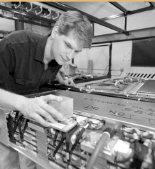
Using an alignment sensor box, Robert Lee checks a muon chamber before shipment to CERN.
