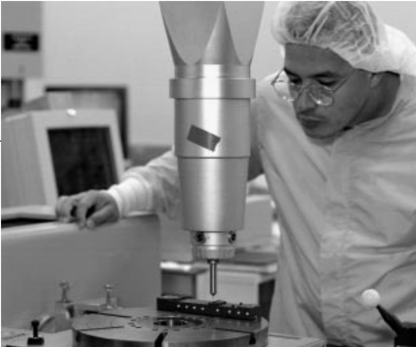
Precision silicon technology has a large role in both detectors' upgrades. Technician Jorge Montes uses a coordinate measuring machine in the Silicon Detector Facility.
